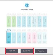
For the example shown, use the 100% IPA option unless you need to change the concentration, in which case use **Edit % IPA** using the keypad. Tap **OK** when you are done.
