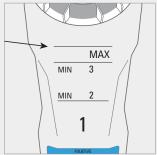
Top off/up the bottle when the reagent is below the minimum level.
