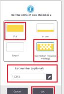
Set the chamber state to Full (molten wax) or Not molten (Parablocks or pellets).
