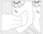
Return the bottle to the cabinet - push firmly into the rear connectors.
