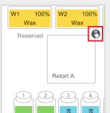
Tap on the retort scanning icon for the retort that is to be used for the protocol run. This opens the retort baskets dialog box.
