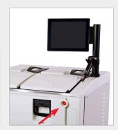
Wait for the screen to go blank, then tap the **power button** at the front of the instrument.
