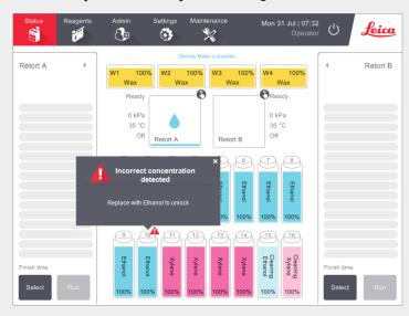
The PELORIS 3 has two density meters, one for each retort. Only ethanol (including reagent-grade ethanol and IPA-ethanol mixtures), IPA and xylene reagents will be checked by the density meters. Fixatives, cleaning reagents and reagent substitutes (such as Histolene) are not checked. Checked Reagents are detailed in the HistoCore PELORIS 3 User Manual (which is located under the Leica symbol on the function bar).
