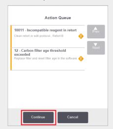
The **Action Queue** window warns you of any actions that are required or recommended before the protocol can be run. Ensure you take note of the message as it also includes steps to take for each code number.
