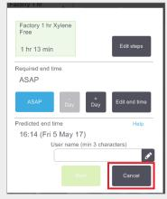
If you realize you have made an error, at this stage you can tap **Cancel**. The edited protocol is displayed on the **Status** screen. From here tap **Unload protocol** to remove and re-load the protocol.
