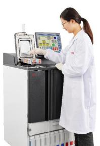
The new ASP6025 S includes magnetic stirrer technology designed to optimize paraffin infiltration performance, helping reduce processing time and enhancing reagent exchange within the tissue cells.
