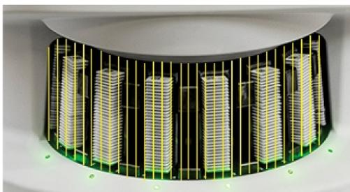
**Figure 6-8:** Pinch points on either edge of rack loading area
