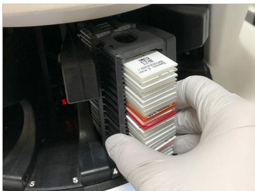
**Figure 6-20:** Rack inserted fully into the carousel
