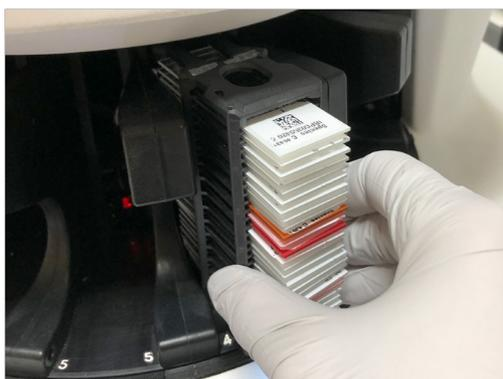
**Figure 6-10:** Rack inserted fully into the rack slot
