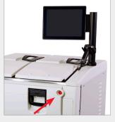
Wait for the screen to go blank, then tap the **power button** at the front of the instrument.
