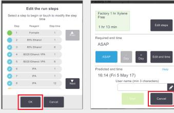
If you realize you have made an error, at this stage you can tap **Cancel**. The edited protocol is displayed on the **Status** screen. From here tap **Unload protocol** to remove and re-load the protocol.
