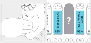
Top off/up the bottle when the reagent is below the minimum level.
