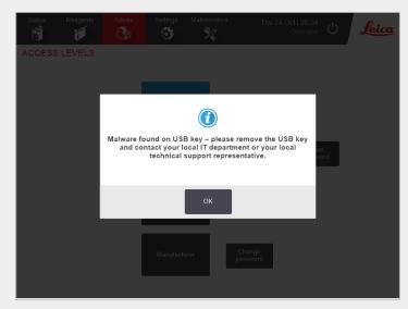
The instrument is equipped with an anti-malware scanner which will scan any inserted USB key. The system will not complete the export or import operation until the anti-malware scan is completed. While the anti-malware scanner is scanning the inserted USB key, the following message will be displayed:
