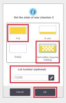
Set the chamber state to Full (molten wax) or Not molten (Parablocks or pellets).
