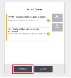
The **Action Queue** window warns you of any actions that are required or recommended before the protocol can be run. Ensure you take note of the message as it also includes steps to take for each code number.
