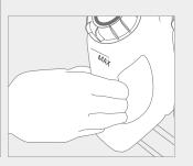
Return the bottle to the cabinet – push firmly into the rear connectors.
