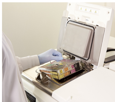
Figure 2-8: Placing a basket into a retort
