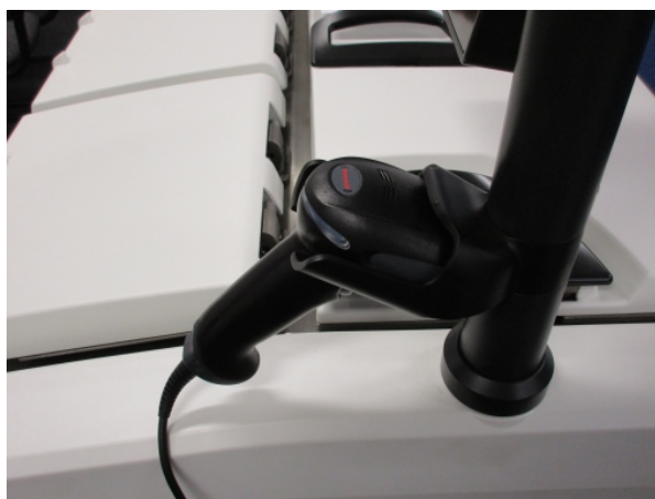
Figure 2-15: Barcode scanner in its cradle
