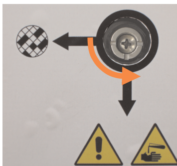
Figure 2-22: Vapor select valve in the external system position
