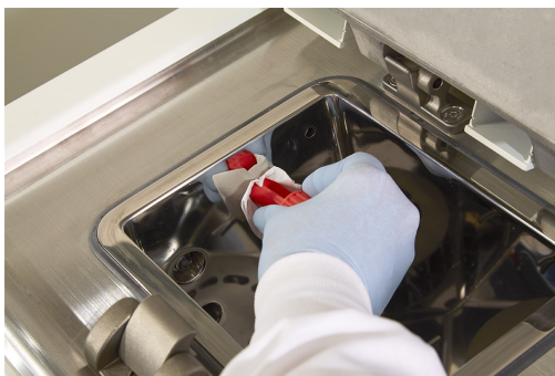
Figure 7-4: Using the LLS cleaning tool
