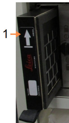
Figure 7-12: Replacing the carbon filter with direction arrow (1) pointing up
