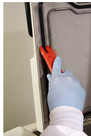
Figure 7-3: Using the wax scraper
