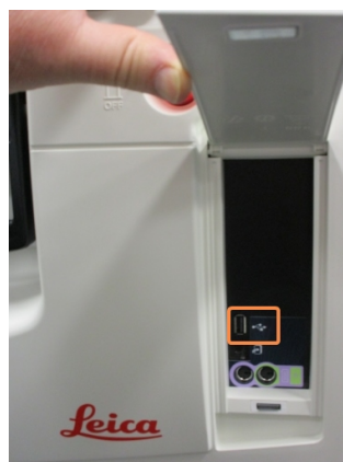
Figure 2-19: Front USB port, behind flap
