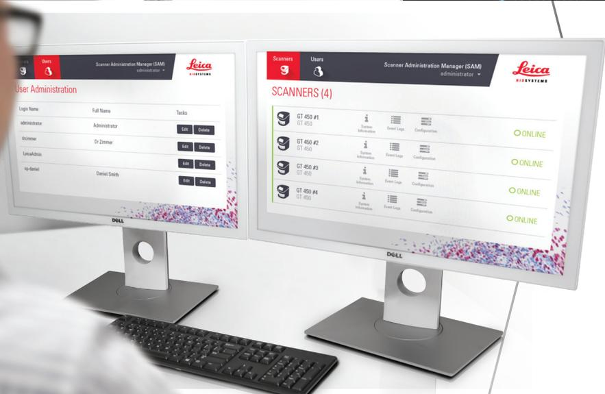
No more workstations needed. SAM server and software allow IT managers to set up and monitor GT 450 scanners via the network, including dashboard status views, PIN controls and log out times.
