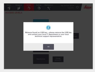
The instrument is equipped with an anti-malware scanner which will scan any inserted USB key. The system will not complete the export or import operation until the anti-malware scan is completed. While the anti-malware scanner is scanning the inserted USB key, the following message will be displayed:
