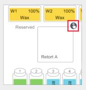
Tap on the retort scanning icon for the retort that is to be used for the protocol run. This opens the retort baskets dialog box.
