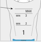
Remove the bottle and safely Fill the bottle to the dispose of the used reagent. maximum level and tighten the cap by hand.
