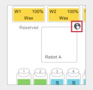
Tap on the retort scanning icon for the retort that is to be used for the protocol run. This opens the retort baskets dialog box.
