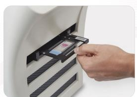
Slide tray eliminates contact with delicate glass slides and remains horizontal at all times
