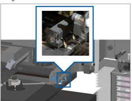
b. Slide the stage to the rear of the scanner, as shown:
