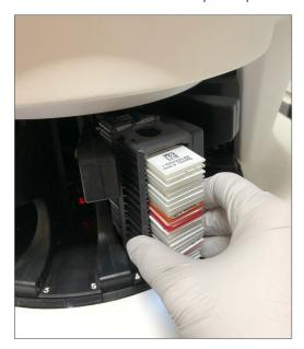
When the rack is fully inserted, there is a "click" sound, and the rack position on the Home screen turns light blue.
