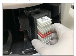
Rack inserted fully into the rack slot:
