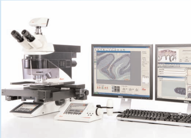
With Leica Microsystems easy-to-use laser microdissection system it is possible to select and cut even single cells from tissue sections.
