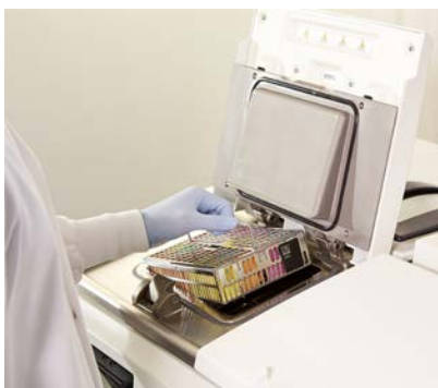
Figure 2-8: Placing a basket into a retort
