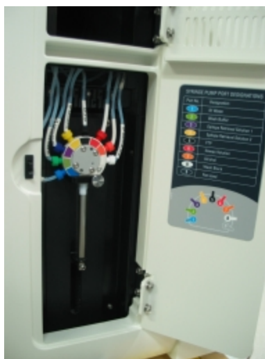
Figure 2-6: Syringe behind hinged door
