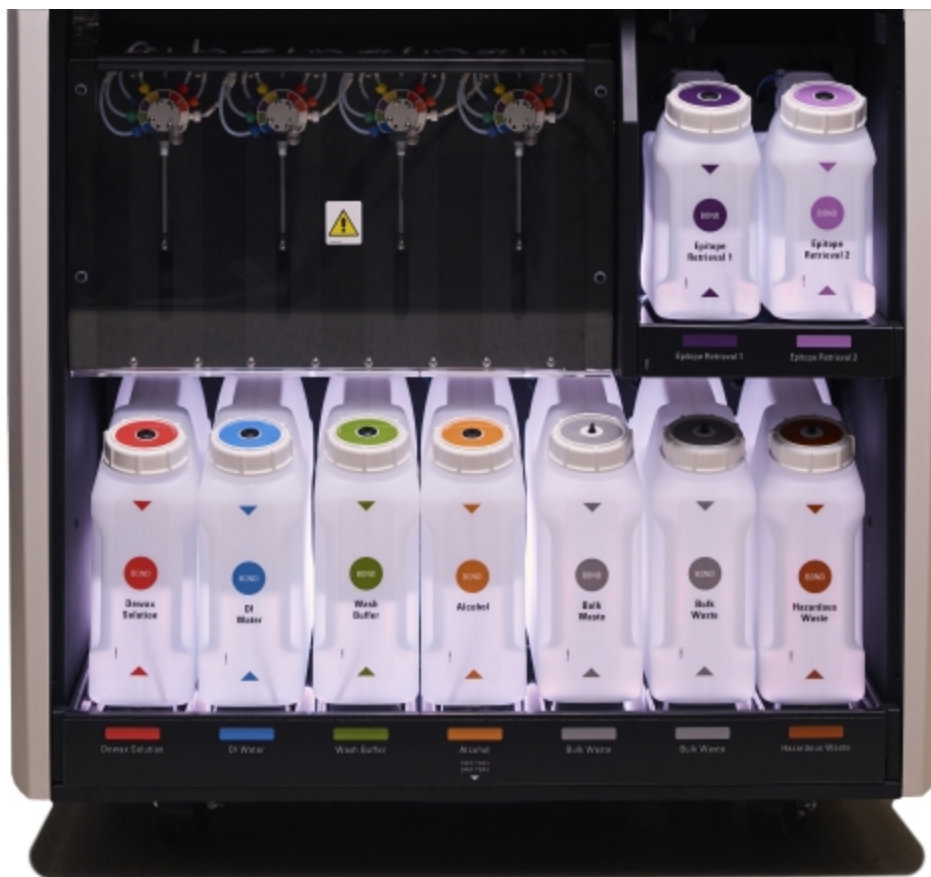
Figure 2-16: Bulk container lighting system
