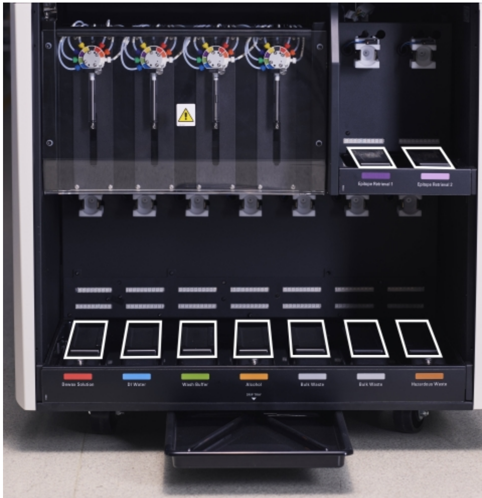
Figure 12-15: BOND-III bulk container drip trays showing the weight sensor covers
