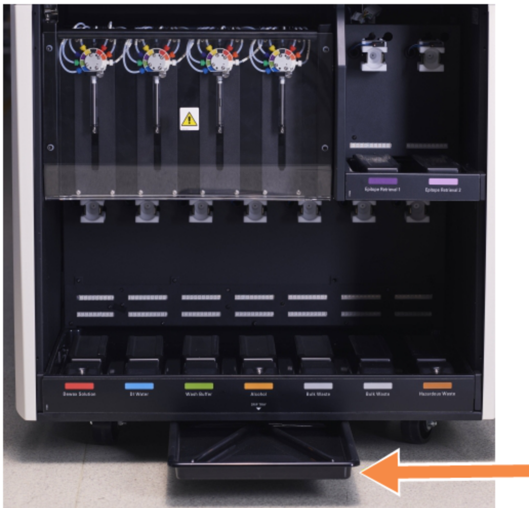
Figure 12-16: The BOND-III instrument drip tray
