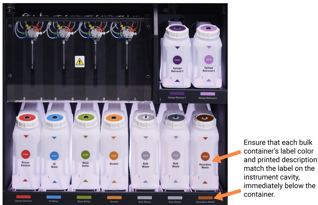
Figure 2-15: BOND-III bulk reagent containers in position
