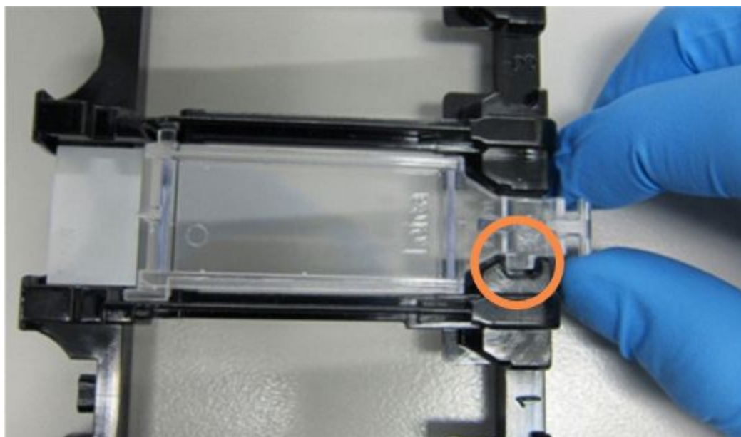
Figure 4-6: Positioning a Covertile on a slide
