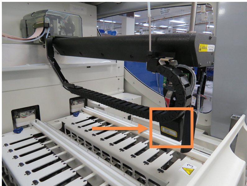
Figure 2-7: Photo of the main robot with the ID imager indicated by the arrow
