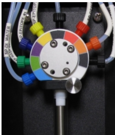
Figure 2-24: BOND-MAX 9-port syringe
