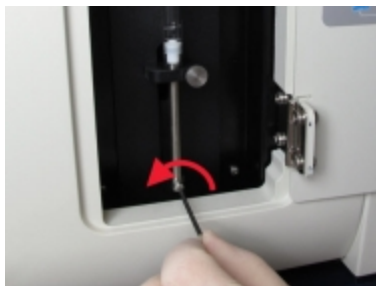
Figure 12-19: Unscrewing the plunger lock screw with a hex key
