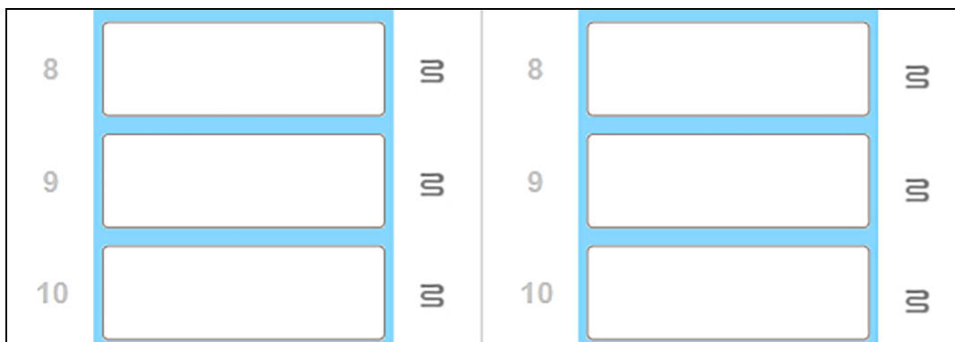
Figure 2-9: Gray heater symbols at each position indicate a complete heating shutdown
