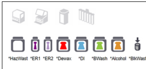
Figure 5-10: Bulk containers (BOND-MAX configuration). The right-most icon represents the external waste container
