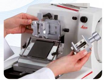
2 Quick exchange specimen clamp
