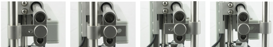
Figure 19. Four positions for attaching the probe shaft to the manipulator
