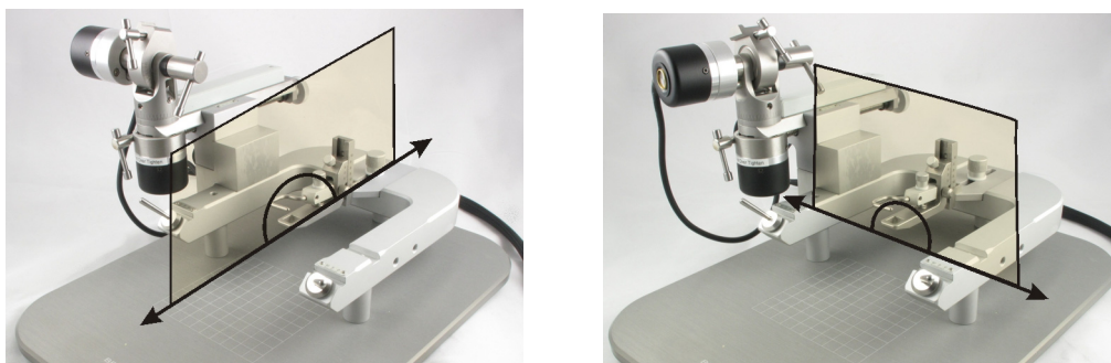
Figure 13. The plane of tilt in the AP and ML directions, showing the tilt range
