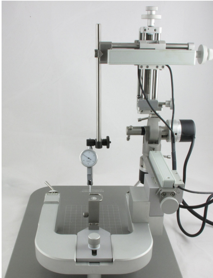
Figure 38. The dial indicator attached to the Angle Two
