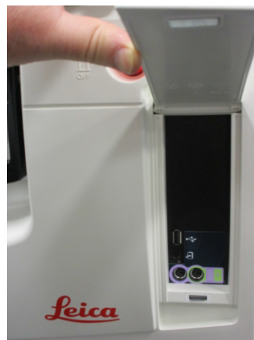
Figur 2.17: USB-port foran bag flappen
