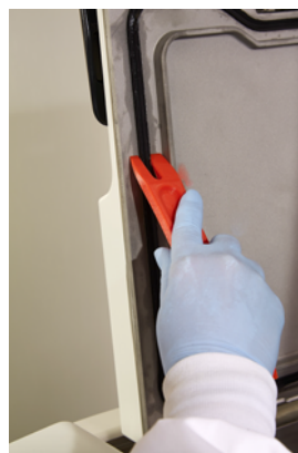
Figure 7.3: Using the wax scraper
