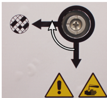
Figure 2.20: Vapor select valve in the internal filter position
