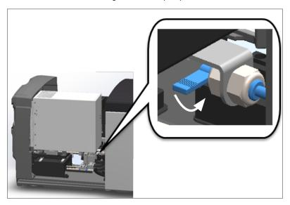
5. Carefully pivot the VPU outward as shown:
