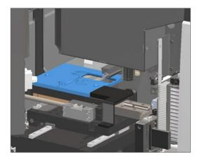
c. Slide the pusher to the front of the scanner, as shown in the rightmost image below. Hold the pusher in one of the areas circled below. Avoid touching the LED and objective.
