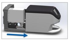
b. Rotate the VPU latch.
