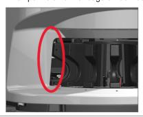
2. Ensure the racks in the rack loading area are inserted correctly:
