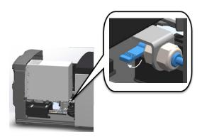
3. Slide the scanner cover back into position so that it is aligned with the rear latches and clicks closed.
