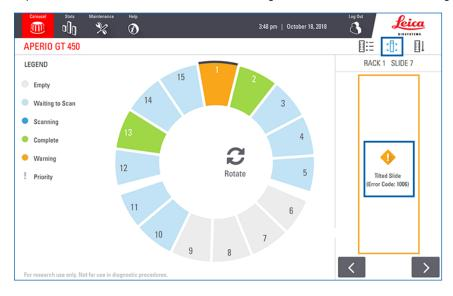
**6.** Take note of the error code and message. For information and steps to resolve the error, go to "Slide Errors and Solutions" on page 70.
