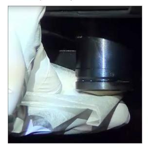
7. With a clean lint-free microfiber cloth, use the same technique described in step 6 to clean the Koehler. The Koehler is located below the objective, as shown circled in white below.
