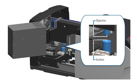
4. Manually position the slide stage so that you have clear access to the objective, as shown below.
