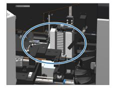
**6**. If possible, carefully remove the slide that is causing the obstruction.
