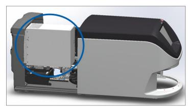
2. Secure the VPU in place by rotating the VPU latch toward you 180 degrees.
