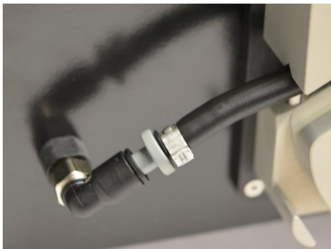
Figure 7-10: Remove Plug from Exit Port
