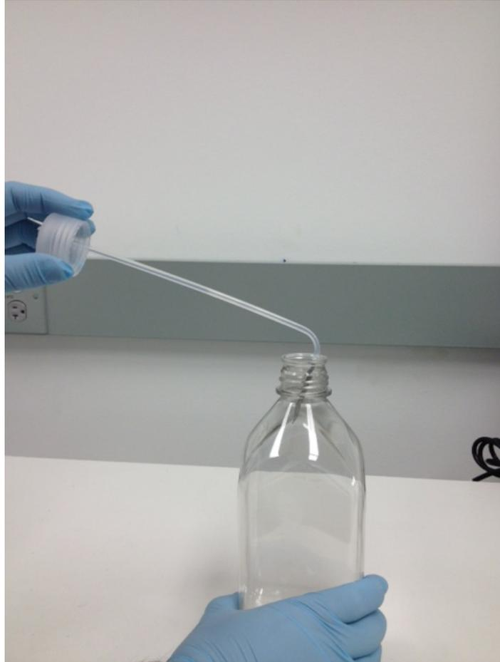
Figure 5-2: Removing Reagent Bottle Caps and Filters
