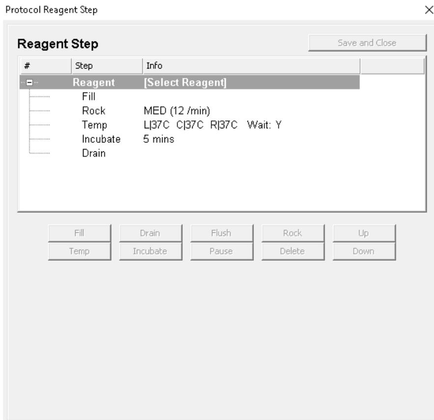
Figure 6-23: Protocol Reagent Step screen
