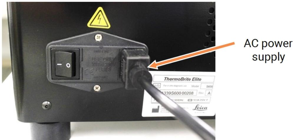
Figure 3-1: Power port located on the back of the instrument
