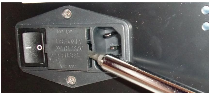
Figure 7-14: Power Switch—Access Fuse Holder
