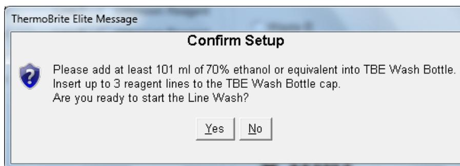
Figure 7-4: Confirm Setup
