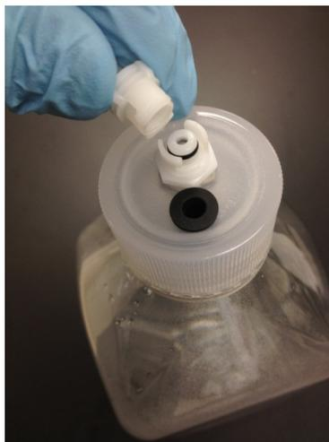
Figure 5-3: Lock Reagent Tube Fitting
