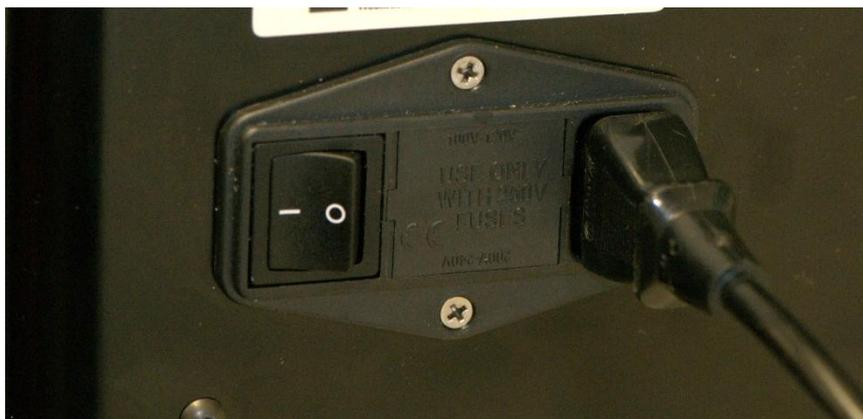
Figure 7-13: Power Switch—Fuse Box
