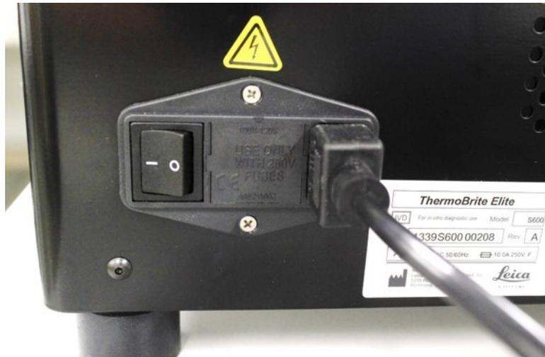
Figure 4-10: Power Switch - It includes the Fuse Box
