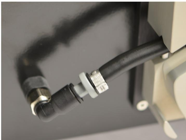
Figure 7-11: Insert Plug into Exit and Inlet Port
