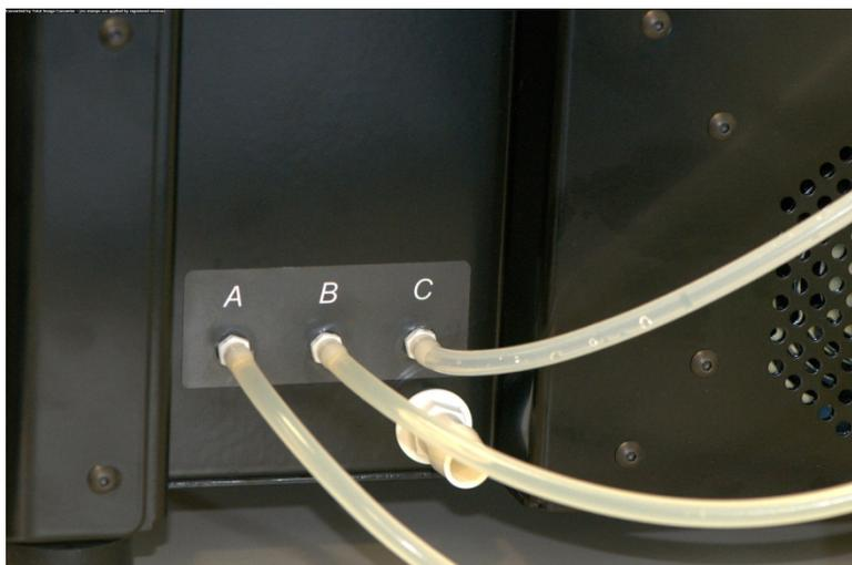
Figure 4-4: Waste ports located on the right side of the instrument
