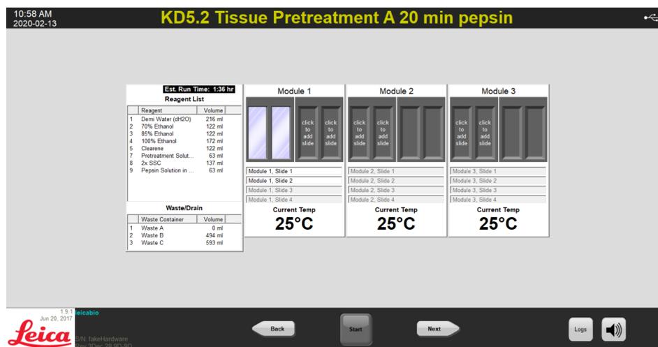
Figure 6-5: Protocol Dashboard—Slide in Sample Chamber
