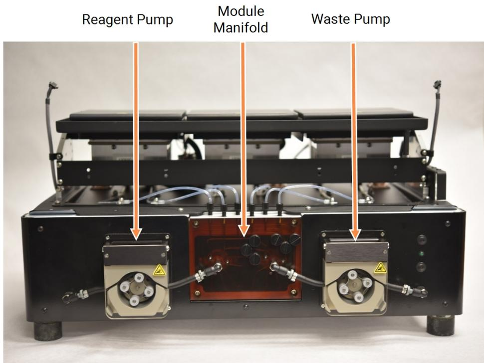
Figure 4-5: Peristaltic pumps located in front of the instrument
