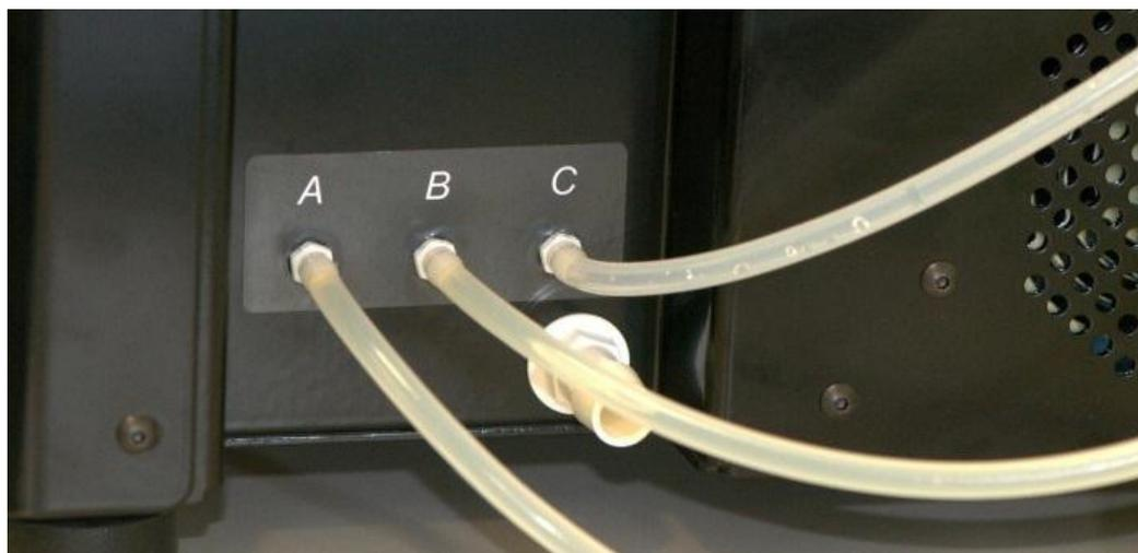
Figure 3-13: Connect Waste Tube to Waste Port
