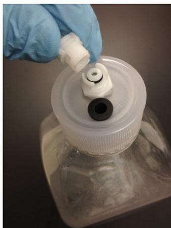
Figure 3-11: Reagent Bottle Cap Fitting
