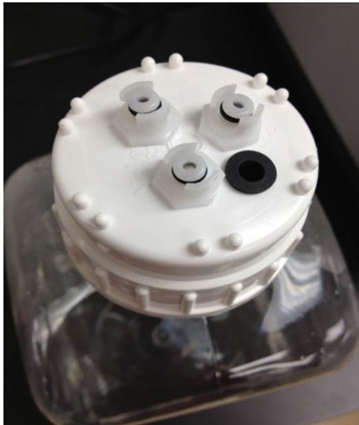
Figure 7-1: Insert Reagent Line Fittings onto Wash Bottle
