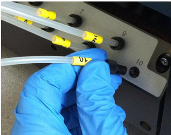
Figure 3-10: Reagent Manifold assembly
