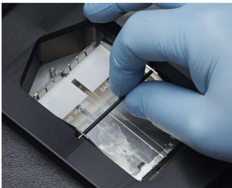
Figure 5-5: Insert Slide Carrier into Sample Chamber
