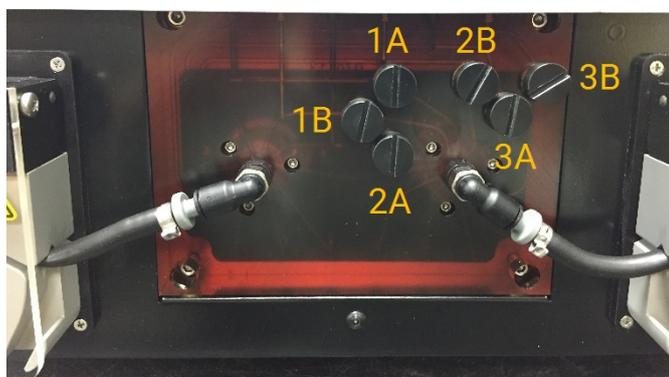
Figure 4-6: Module Manifold
