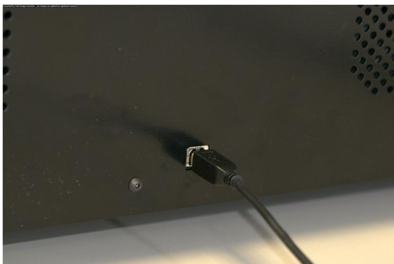
Figure 3-4: Communication port located in the center of the back panel
