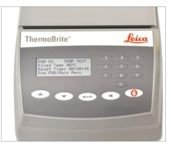
This programmable system automates the denaturation and hybridization steps in slide-based FISH procedures, and provides walk-away convenience for clinical and research personnel. The low cost unit accepts a wide range of sample types, is easy to use, and reduces hands-on time by more than 50% while ensuring overall precision and accuracy in FISH assays.
