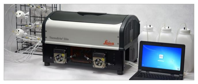
The ThermoBrite Elite automates and standardizes the FISH slide preparation process including deparaffinization, pretreatment, denaturation/hybridization and post hybridization wash.
