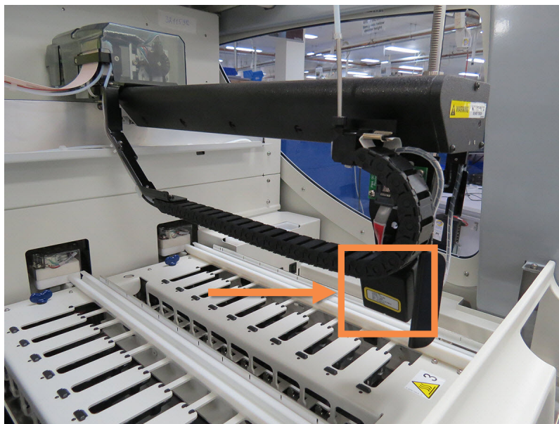
Figure 2-6: Photo of the main robot with the ID imager indicated by the arrow
