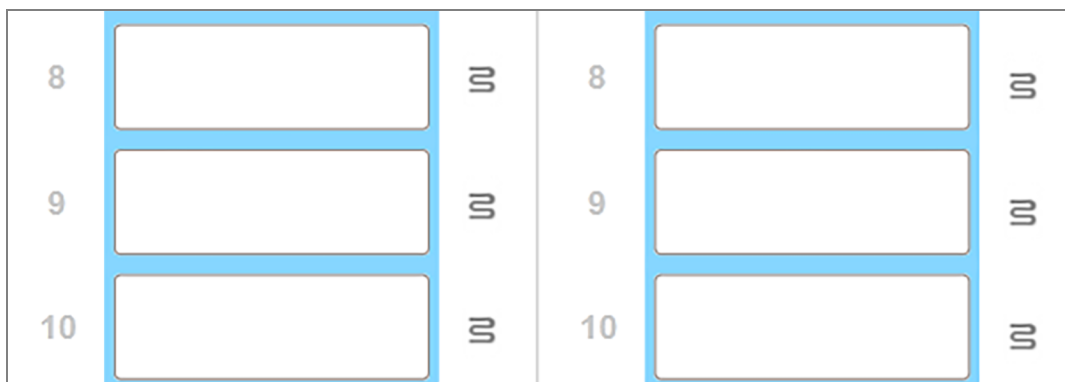
Figure 2-8: Gray heater symbols at each position indicate a complete heating shutdown
