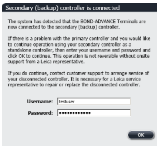
Figure 16-6: Dialog - secondary (backup) controller connected
